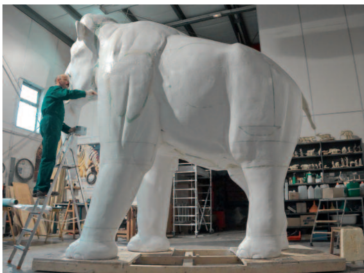
Stratification du mannequin © MNHN/B. Faye
